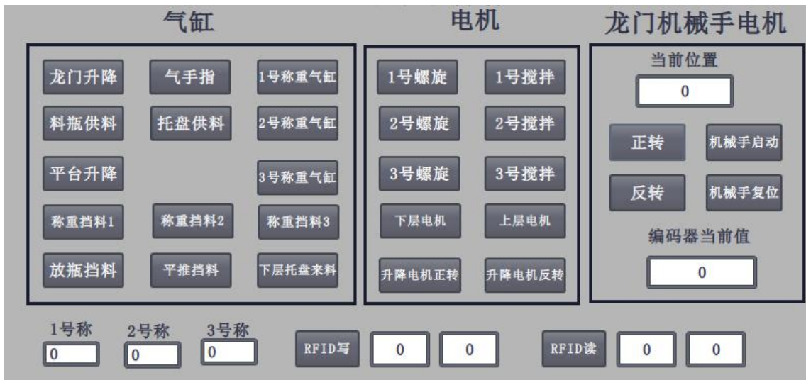
Fig. 2-2 Manual Operation Page of Feeding and Filling Station
