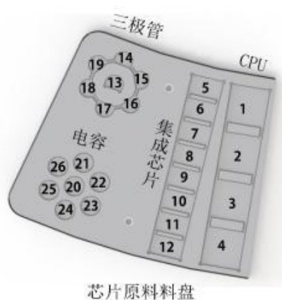
Figure 4-3 Location number of material plate chips
