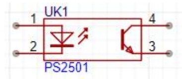
Figure 1 Drawing of optocoupler style
